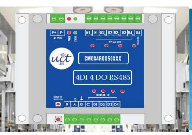
4 Digital Input 4 Digital Output to RS485 converter module converts the 4 digital input and 4 digital output data to RS485.
