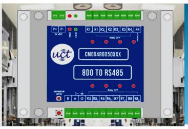
The 8-Digital Output to RS485 Modules converts input from connected Modbus Master over RS485 to digital output
